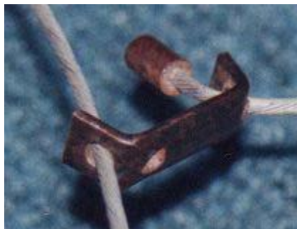
A close up of the metal bracket on the same snare - note that the wire is threaded through the outermost of the two holes in the bracket
