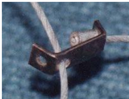
A close up of the metal bracket on another dual-purpose snare. Here, the wire is threaded through the innermost of the two holes in the bracket. This makes the snare a free-running snare
